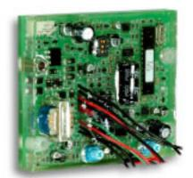
Standard practice for manufacturing emergency phones is to provide them with standard uncoated circuit boards (like the ones in your PC). A few manufacturers, including Viking, spray the circuit boards with a water resistant material such as acrylic conformed coating to protect them.
